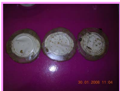
Figure 3. Chemcatcher (inorganic version)
